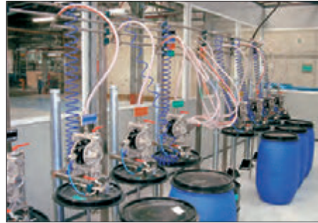
1/2" diaphragm pumps installed in a coloring process
