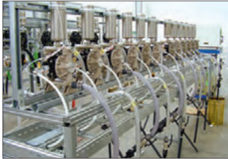
1/2" diaphragm pumps assembled in an ink formulation system
