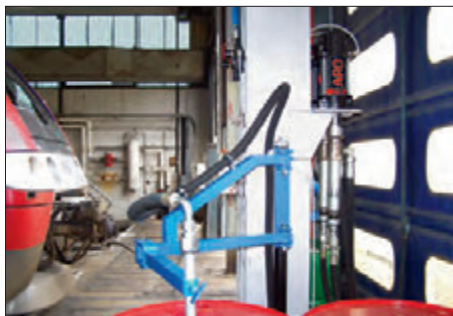
2-ball piston pump 9:1 ratio, used in a customized lubrication process
