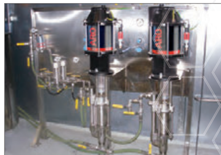
4-ball piston pumps, 4:1 ratio, installed on a paint formulation system process
